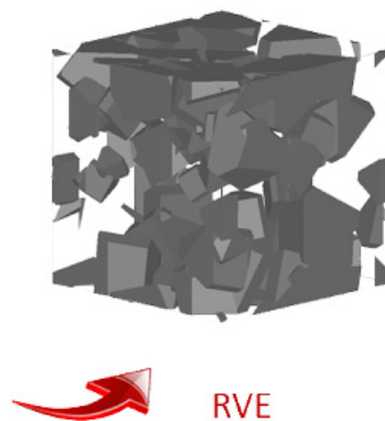
Generation of complex RVE based on geometric shape & size distribution
